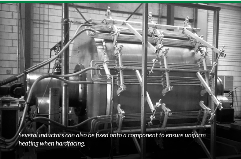
Heating from the outside with fixed inductors of rotating pipes.
