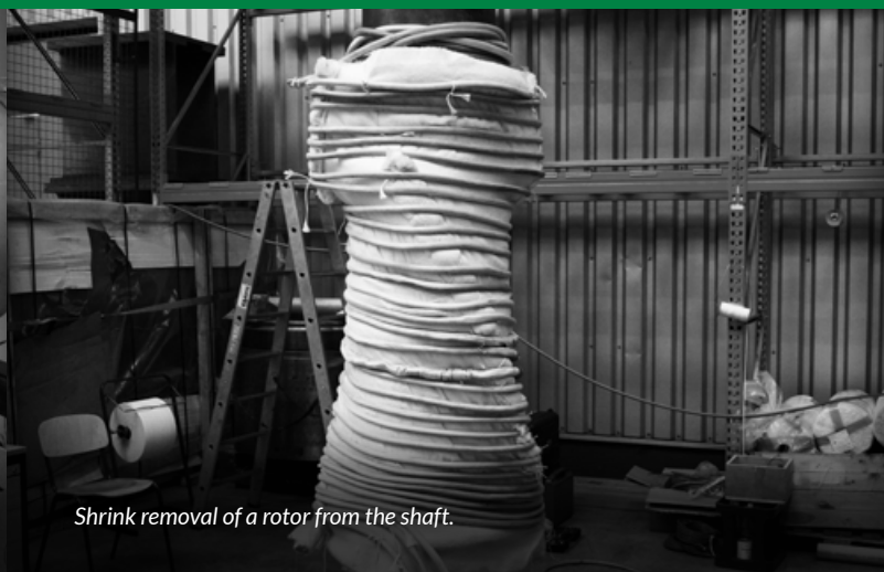
Flexible coil inductors are especially suitable for preheating or stress-relieving of pipes or other components.
