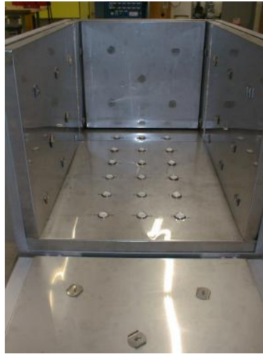
Preheating- and Annealing boxes for the preheating and stress relieving of tools and forging dies
